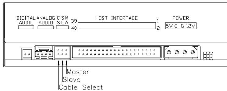
If you connect only one device on the cable, you can set the jumper as "master" or "slave".
